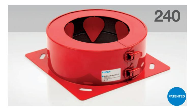
Valsir Collarwings 240 is the new range of fire stop collars produced in compliance with the most recent standards and suitable for installation on plastic waste and drainage pipes. The Collarwings 240 fire stop collars are made of steel and painted with polyester powder fitted with special intumescent inserts which, in the event of fire, expand and squeeze the pipe thus preventing the passage of flames, combustion gas and vapours and acting as a thermal insulation.
