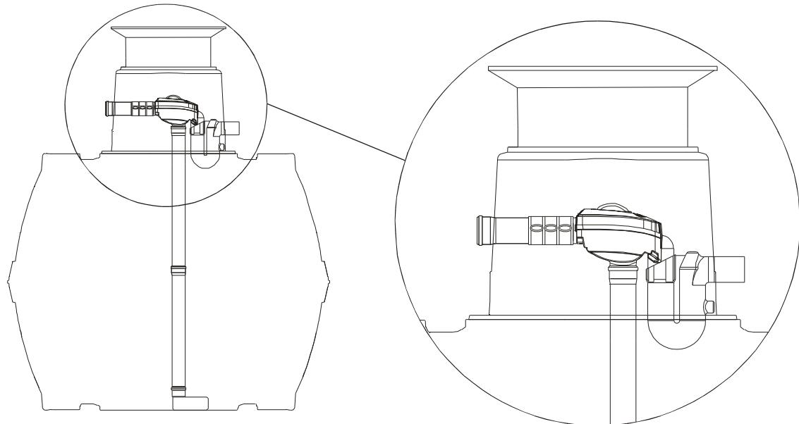
Insert the filter, prepared with the inflow pot (calmed down), in the tank.
