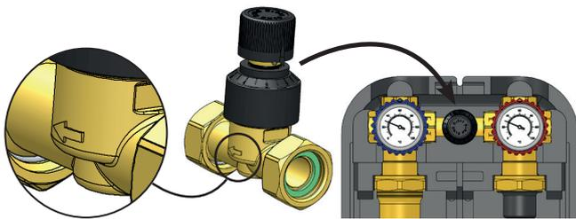
**Heat metering:** 23G.DN25 groups are equipped with specific extension to install energy metering devices, G 3/4 110 mm or G 1 130 mm. They are also complete with pocket for immersion temperature probe on the red knob monobloc.
