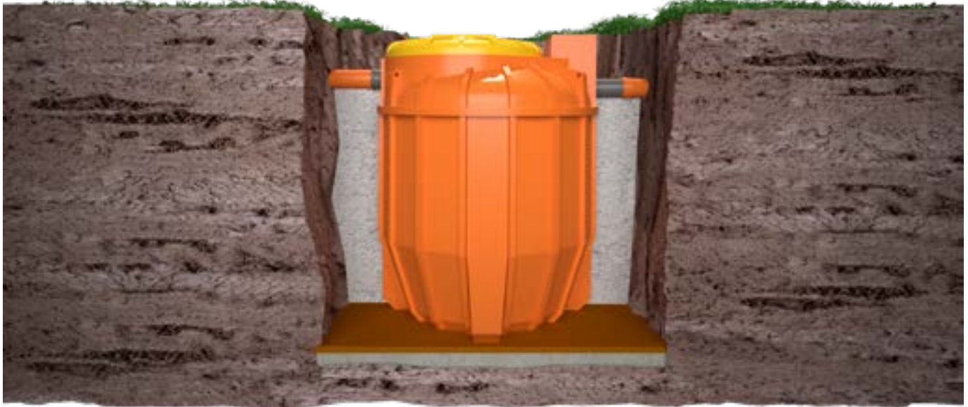
Figure 5.5 Laying with surface water table.
