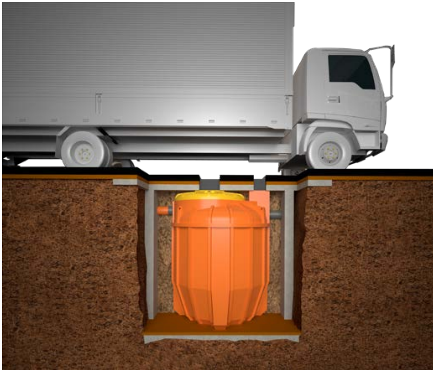
Figure 5.11 Heavy vehicle access - class D 400.
