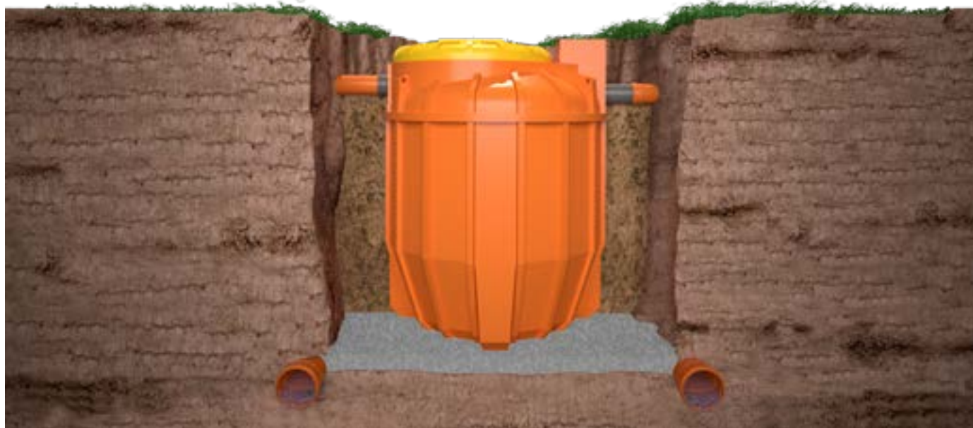
Figure 5.6 Laying with clayey soil.
