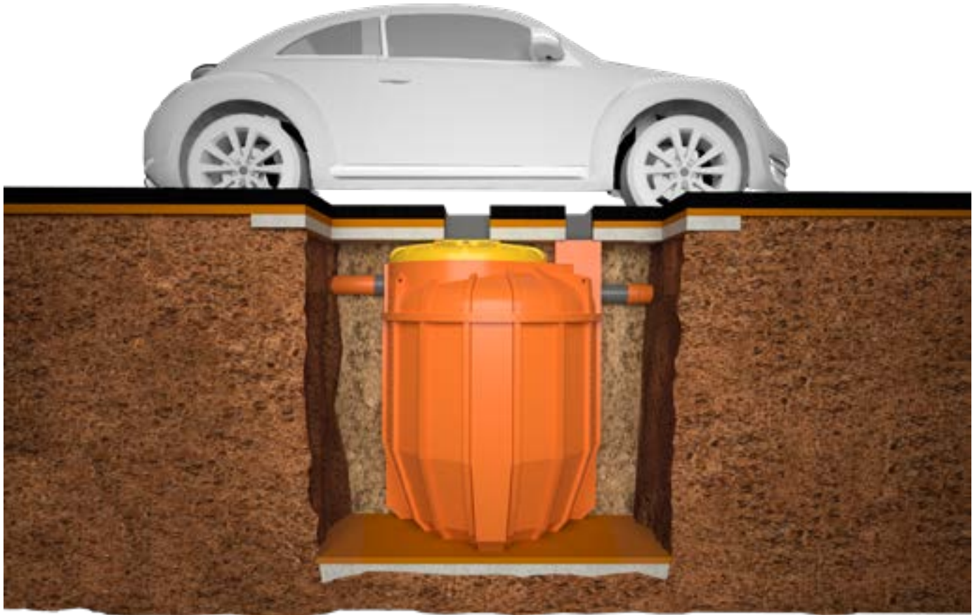
Figure 5.10 Light vehicle access - class B 125.
