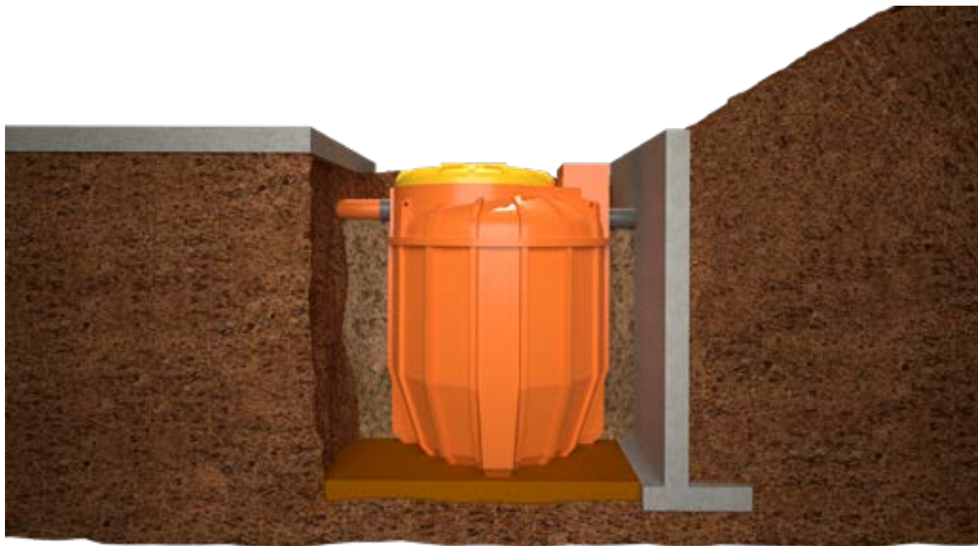
Figure 5.8 Laying near a slope.
