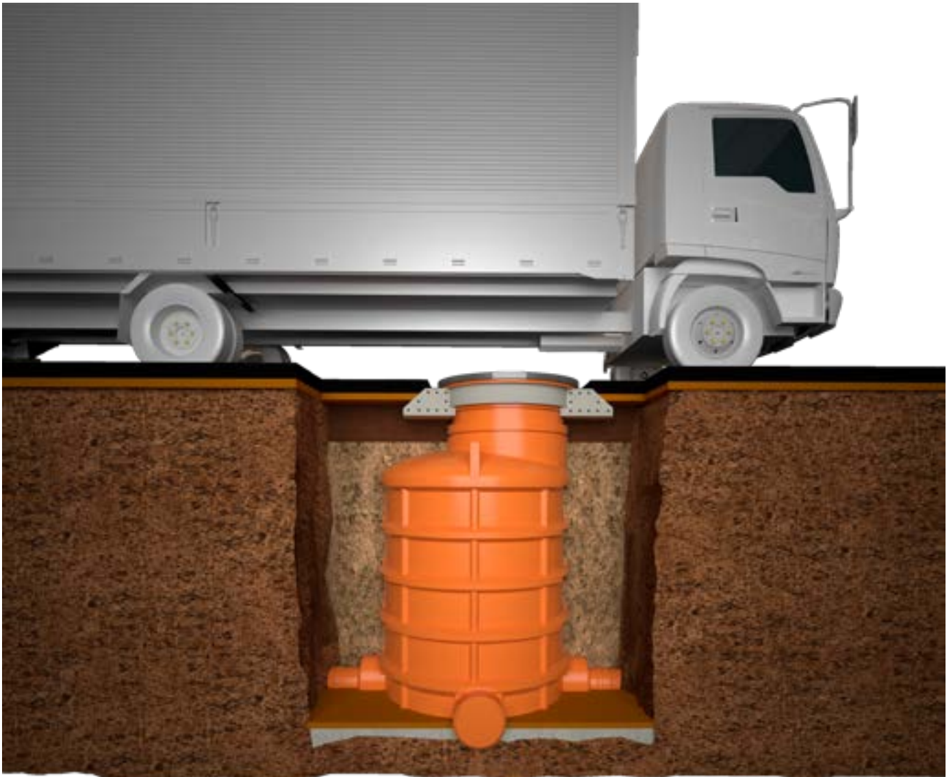
Figure 5.12 Laying with concrete ring to distribute external loads.
