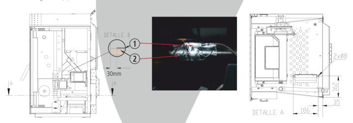
Measurements and example of location of the NTC for the Cantina Compact model. The NTC will be set the same as in the HIDRO.
